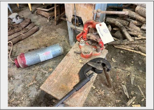
**Description** Pipe Vise With Pipe Cutter **Quantity:** 1
